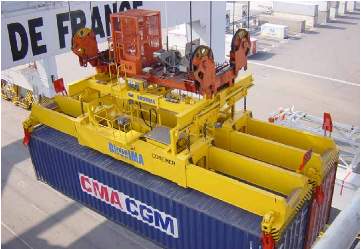
Tandem E 3 is the new twin lift spreader from Bromma. It is spreader optimized to meet the productivity requirements from the new mega vessels.
