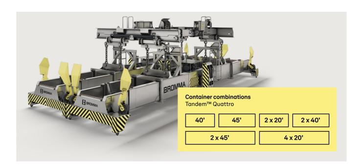
The Tandem™ Quattro is a highproductivity, lower weight Tandem™ solution. The limitation on Tandem™ Quattro is that it is not designed to lift a single 20' container. The Tandem™ Quattro is especially well-suited for container terminals that have a high percentage of 40' and 45' containers, and a low percentage of 20' containers that are located in such a way that they need to be loaded/ unloaded in single lift mode.
