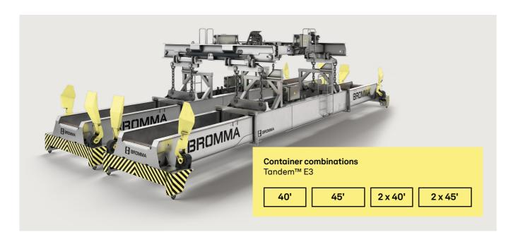
The Bromma Tandem™ E3 spreader offers great capacity and flexibility. Low spreader weight is combined with the ability to lift different combinations of 40' or 45' containers side by side as shown below. The spreader can also lift single 40' and 45' containers.
