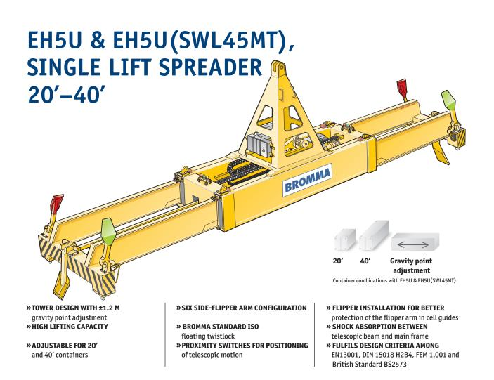
The Bromma EH5U spreader is a single lift mobile harbour crane spreader with high lifting capacity combined with low weight. This means better performance with no impact on the load curve or the travelling of the crane. The EH5U comes with the Bromma standard ISO floating twistlocks with a floating capacity of 6 mm and both electrical interlock and mechanical blockading.
