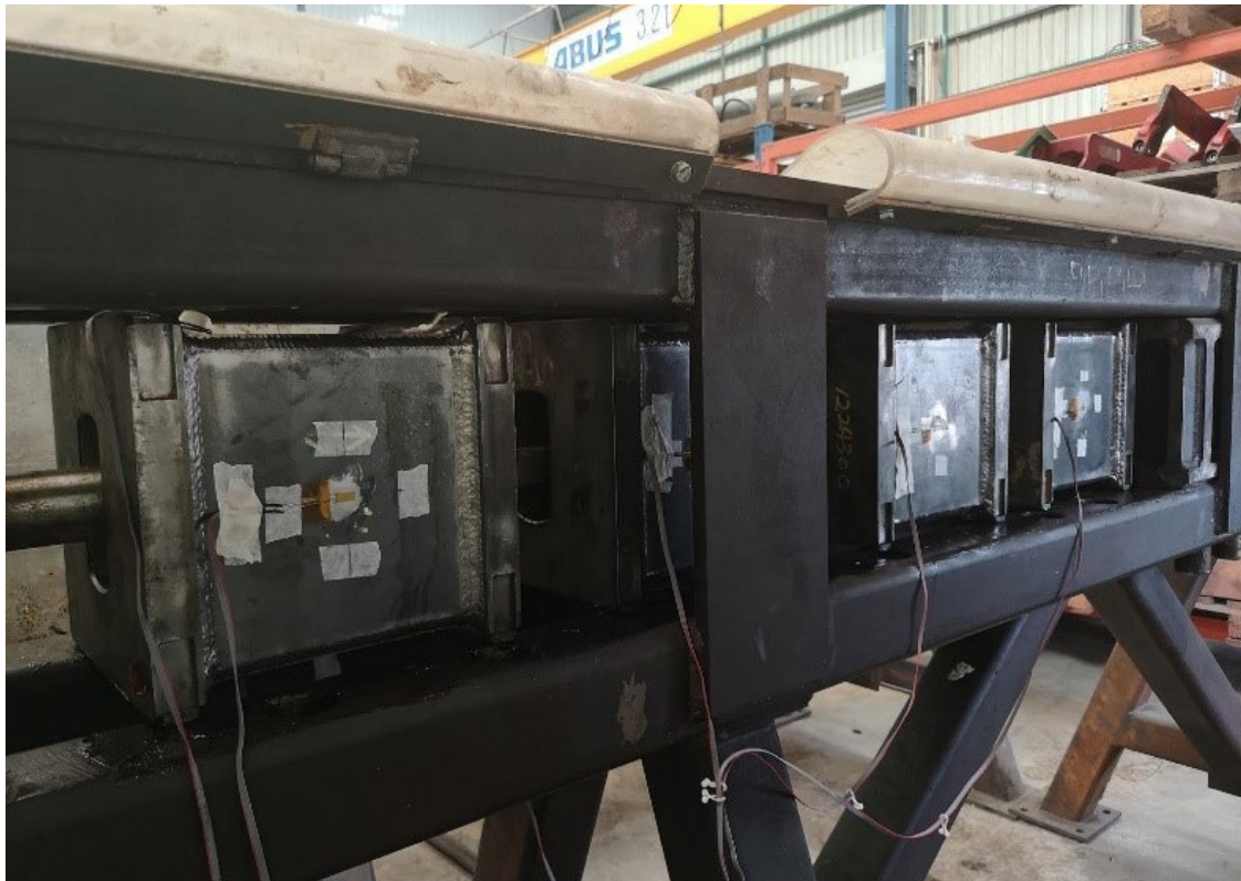
Figure 4. Fatigue testing of box welded structure
