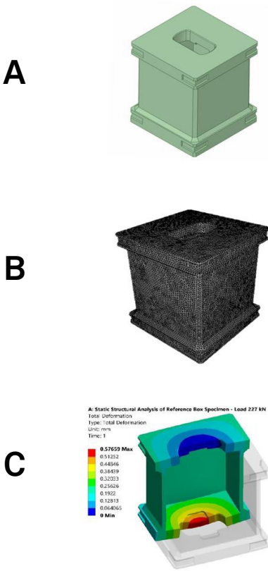
Figure 6. A) Box welded structure, (B) Meshed, (C) Deformation plot
