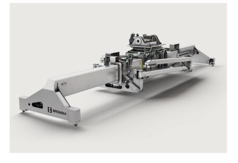
The Bromma RSX40C is a combined reach stacker spreader for single container and trailer handling. It has four grapple arms to lift trailers, swap bodies (C715, C745) and bottom lifting containers.
