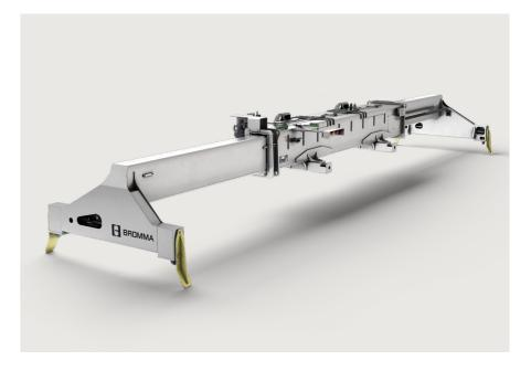
The Bromma TLG40 is a telescopic spreader designed to handle single 20' and 40' containers for masted lift trucks fitted with a gantry and is designed to attach to the truck gantry with 4 telescopic hangers that is selflevelling.
